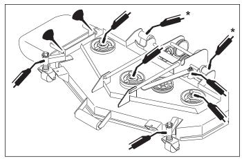
Figure 20. Deck Lubrication
